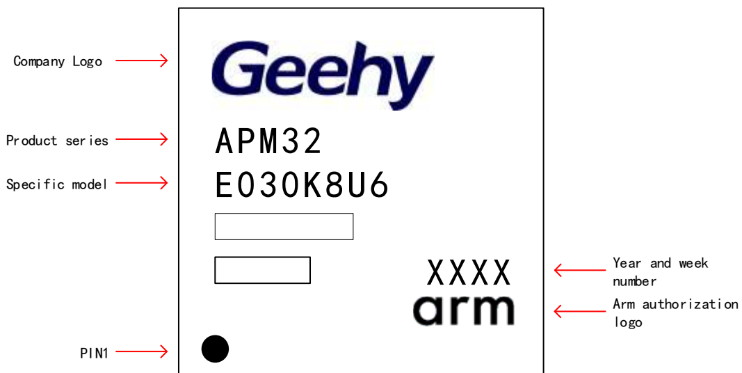
Figure 34 QFN32 - 32 Pins, 5 x 5mm Package Schematic Diagram
